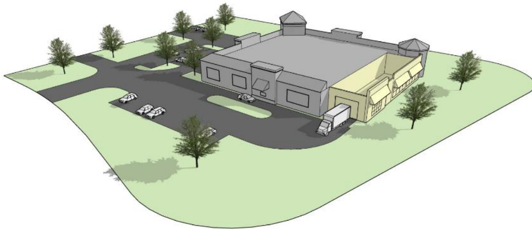
Figure 156.E.007-1 Illustrative Example of Enclosed Loading
